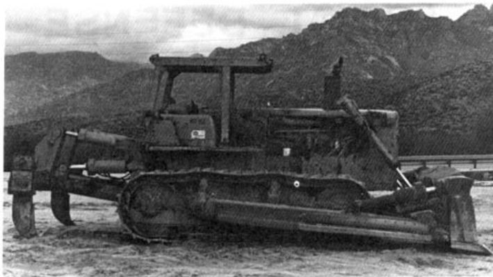
Bulldozer. Note the smoke stack (exhaust pipe).
